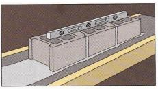
**3.** Check for level and plumb every three blocks. Tap blocks into mortar with trowel to make adjustments.
