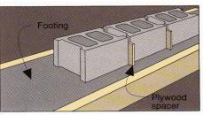
**1.** Before mixing mortar, dry lay first course on footing. Use wood strips for joint spacing. Mark spacings on footing.
