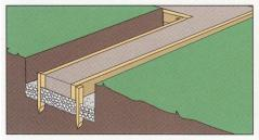
**4.** Coat forms with old motor oil for easy removal later. Pour concrete to top of forms.
