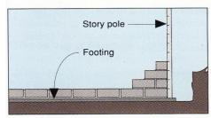
**4.** Build corners or ends after first course. Check with level and story pole. If off, pull blocks and start again.
