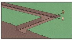
**1.** Stake out lines for the wall. Dig a trench twice the width of the footing. First wall courses will be below grade.
