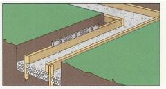
**3.** Stake the forms, making sure they are perfectly level and square. Drive stakes on the outside of the forms.
