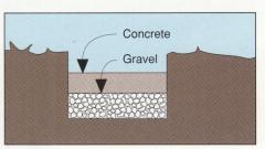
If the ground is hard, you can pour concrete without forms. Dig a straightsided trench the width of the footing.
