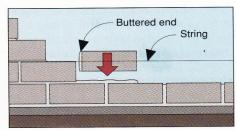
**6.** Lay blocks between corners level with line. Lift blocks into position; don't slide them. Alternate block joints.
